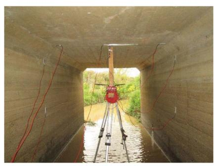
Figure 45: Photo showing the sensors installed in the exterior cell of the culvert
