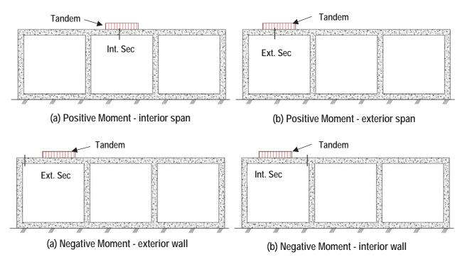
Figure 30: Positioning of Tandem loading to produce maximum positive and negative moments at midspan and wall sections of the exterior and interior cells
