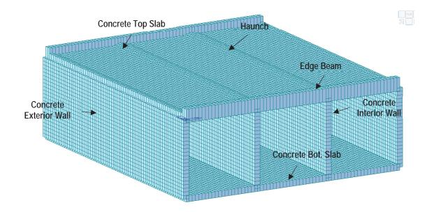
Figure 48: Typical 3D model for the tested culverts
