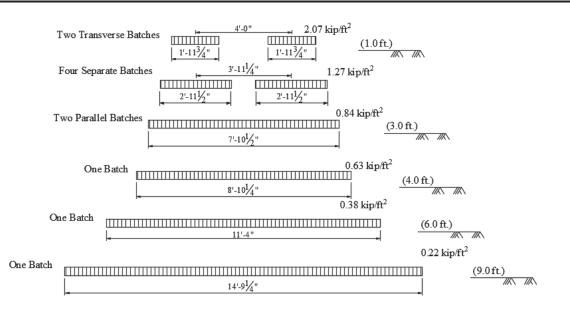
Live load distribution at the surface of the top slab in the direction parallel to span for 10 x 10 culverts
