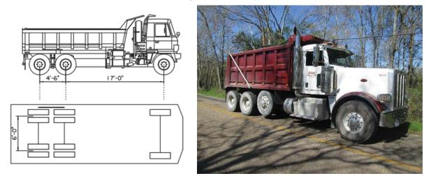
Figure 46: Three axle dump truck used in the testing
