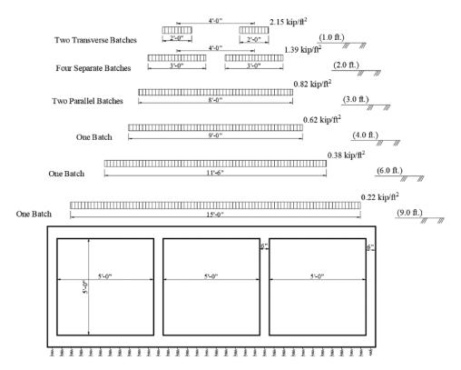
Live load distribution at the surface of the top slab in the direction parallel to span for 5 x 5 culverts
