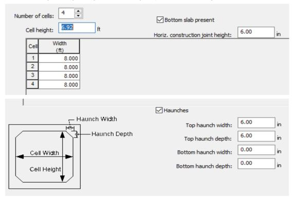
Figure 56: Adjustment of the clear height of the culvert in Bridge Rating Software
