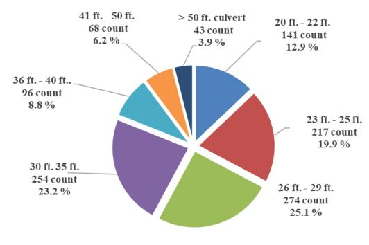
Figure 22: Classification based on the total width of the culvert
