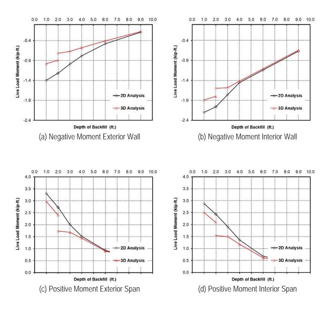
Figure 35: Live load moment from 2D and 3D models for 5X5 culverts
