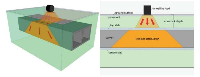
Figure 9: Illustration of live load distribution for RC box culverts (Wood et al., 2016)
