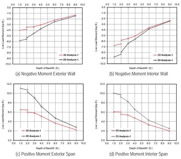
Figure 39: Live load moment from 2D and 3D models for 12X12 culverts
