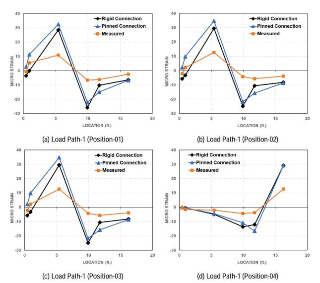
Figure 50: Strain profiles along the top slab of culvert #004360 from the field test and FE models
