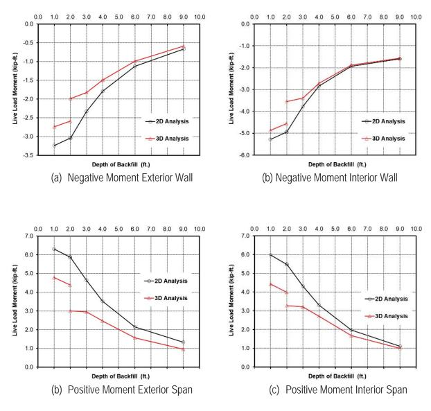
Figure 37: Live load moment from 2D and 3D models for 8X8 culverts
