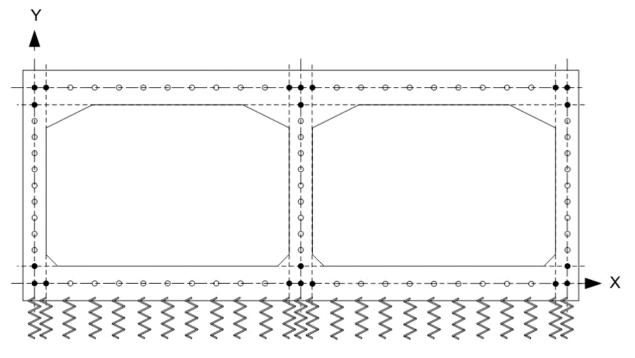
Figure 53: 2D Frame element model in Bridge Rating
