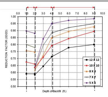
Figure 41: Development of formulas for the correction factors
