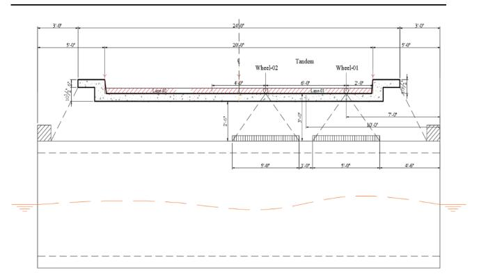
Live load distribution at the surface of the top slab in the direction perpendicular to the culvert span for fill height of 3.0 ft
