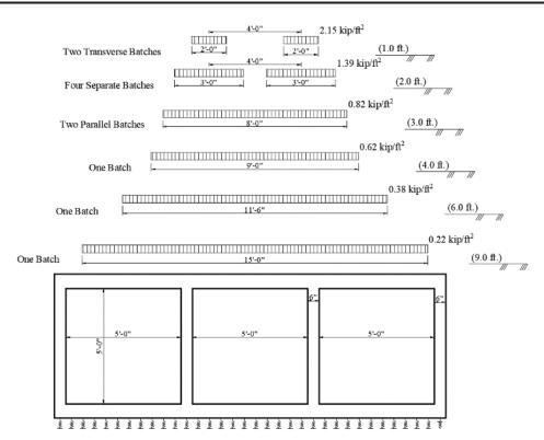
Figure 32: Live load distribution at the surface of the top slab in the direction parallel to culvert span for different fill heights
