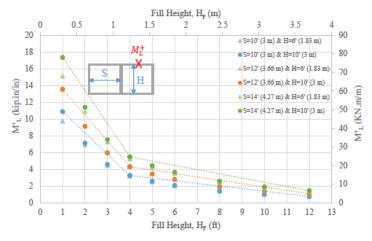
Figure 13: Effect of fill height on the positive bending moment due to live load (adopted from Acharya (2012))
