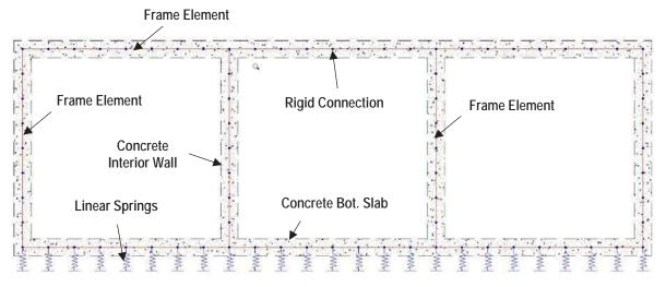
Figure 27: Schematic representation of the 2-D frame element model
