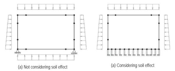
Figure 15: Consideration of soil effect in two-dimensional frame-element structural models
