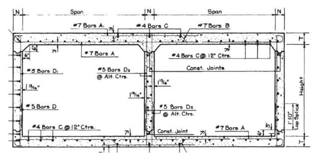
Figure 3: LADOTD standard reinforcement details of double-cell RC box culvert in Louisiana DOTD
