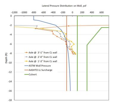
Figure 11: Live load surcharge pressure on culvert wall against backfill depth (adopted from NCHRP 15-54)
