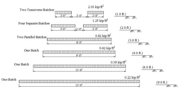
Live load distribution at the surface of the top slab in the direction parallel to span for 12 x 12 culverts
