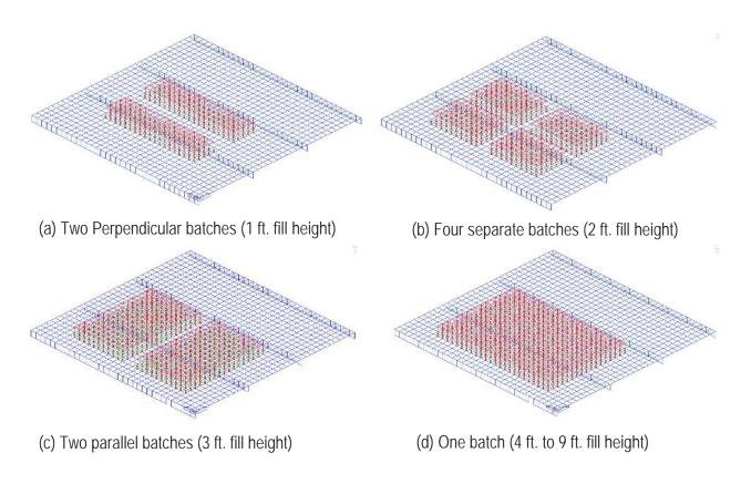
Figure 31: Live load configurations at the surface of the top slab
