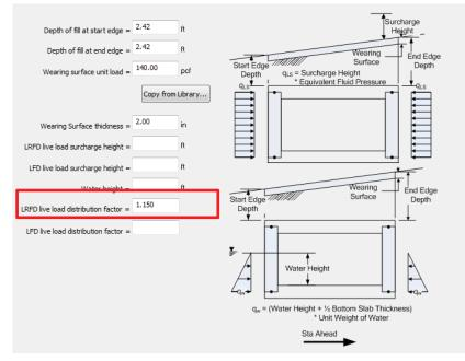
Figure 62: Adjustment of the live load distribution factor in BRr software
