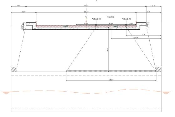
Figure 33: Truck positioning in the direction perpendicular to culvert span
