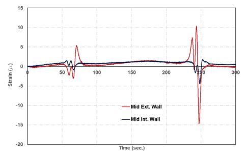
Figure 52: Strain at the mid height of the exterior and interior walls during dynamic test, RC# 004360
