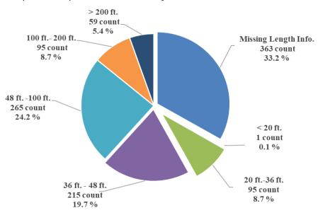
Figure 24: Classification of the inventory based on length of culvert
