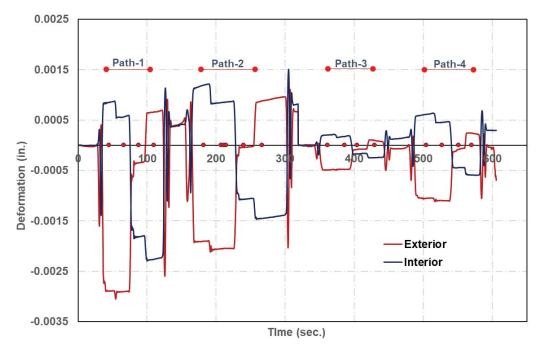
Vertical displacement at midspan of exterior and interior cells during static loading of Culvert
