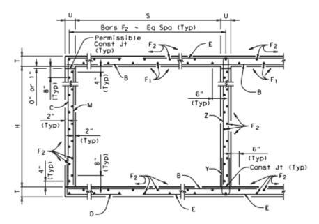
Figure 4: Texas standard reinforcement details of multi-cell RC box culvert in Texas DOT
