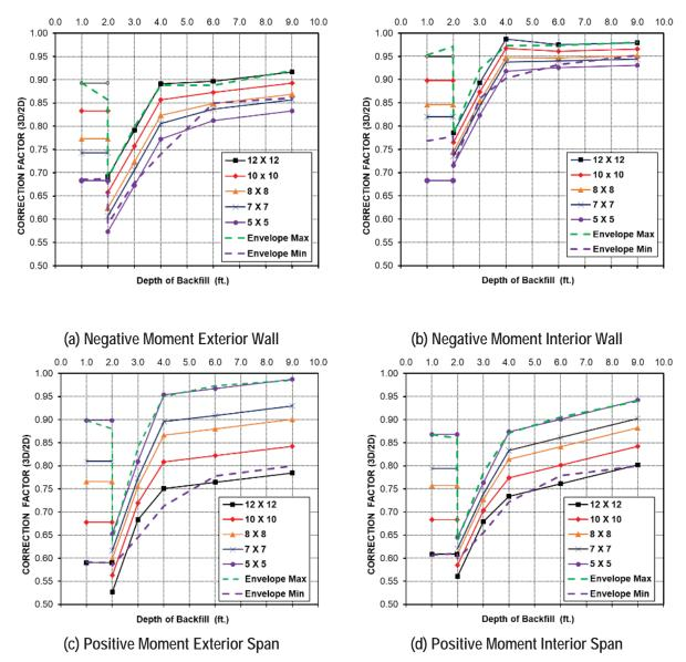
Figure 42: Correction factors between 3D and 2D models for culvert with different sizes
