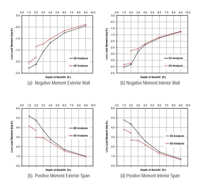
Figure 36: Live load moment from 2D and 3D models for 7X7 culverts
