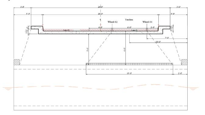
Live load distribution at the surface of the top slab in the direction perpendicular to the culvert span for fill height of 6.0 ft
