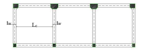
Figure 57: Rigid parts that need be extracted from culvert span length
