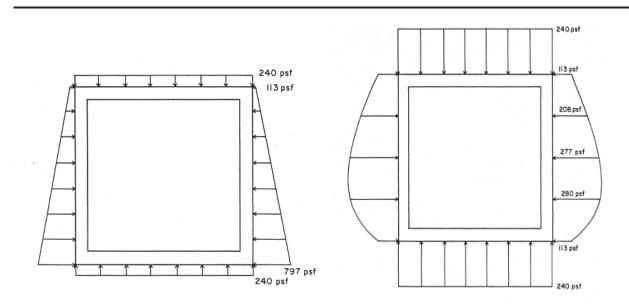
Figure 6: (a) at rest linear distribution for the lateral soil pressure (AASHTO) on culvert exterior wall and (b) measured nonlinear distribution for the lateral soil pressure due to soil arching effects.
