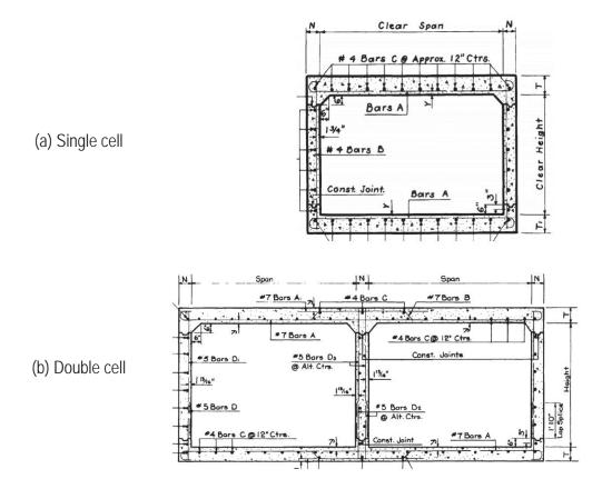
Figure 1: LADOTD standard reinforcement details of single- & double-cell RC box culvert
