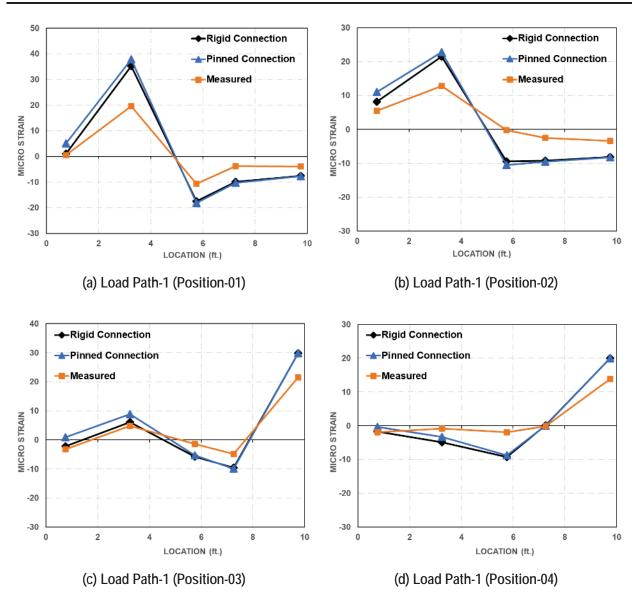
Strain values at the top slab of culvert from field measurements and FEM models
