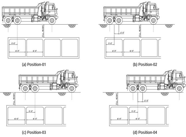
Figure 47: Loading positions for each loading path
