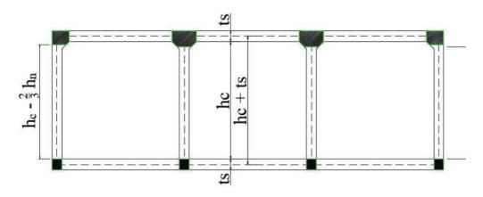
Figure 55: Rigid parts that need be extracted from culvert height
