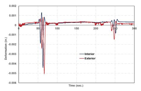
Figure 51: Deformations at midspan of exterior and interior cells during dynamic test, RC# 004360
