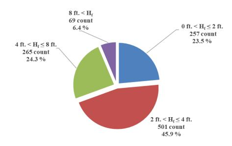
Figure 23: Classification of the inventory based on height of backfill
