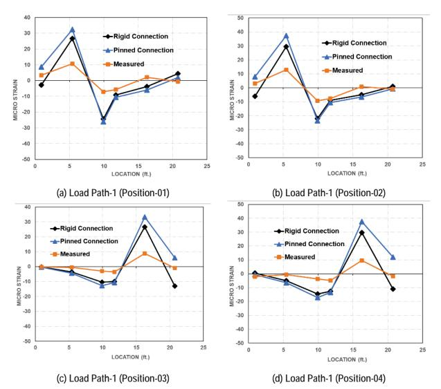
Strain values at the top slab of culvert from the field measurements and FEM models
