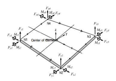
Figure 28: Nodal forces for the plate element
