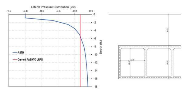
Figure 63: Live load surcharge from ASTM standards versus AASHTO LRFD
