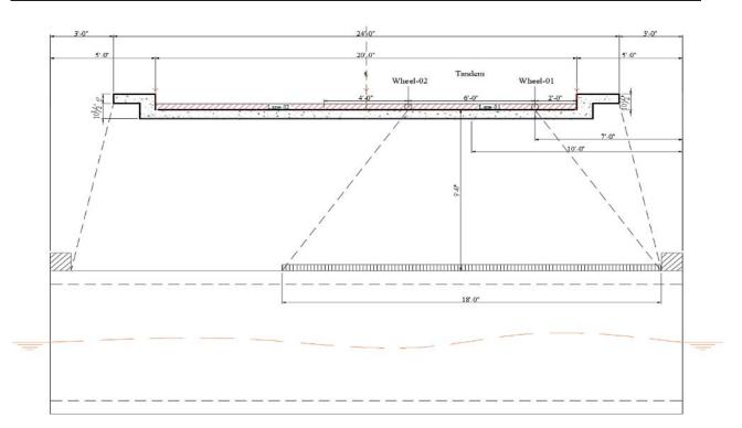
Live load distribution at the surface of the top slab in the direction perpendicular to the culvert span for fill height of 9.0 ft
