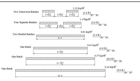
Live load distribution at the surface of the top slab in the direction parallel to span for 7 x 7 culverts
