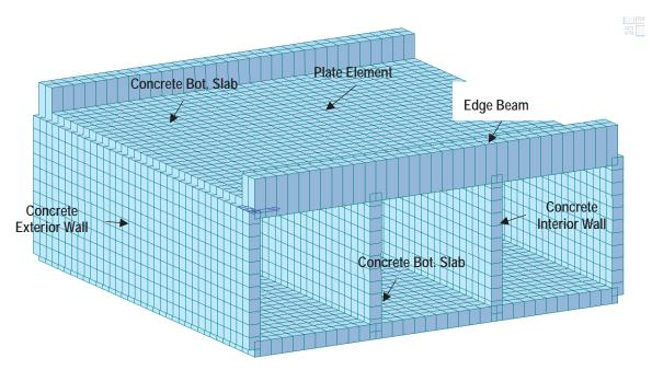
Figure 29: Typical 3-D shell element model
