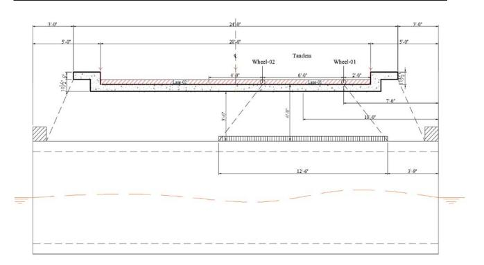
Live load distribution at the surface of the top slab in the direction perpendicular to the culvert span for fill height of 4.0 ft
