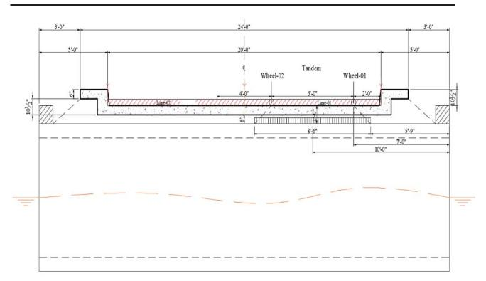
Live load distribution at the surface of the top slab in the direction perpendicular to the culvert span for fill height of 1.0 ft
